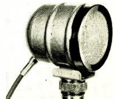
rat-tail file, and a disc cut from fine-mesh wire screen has been cemented to the lid.—Art Trauffer R-E
