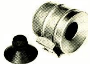
A photo shows the completed mike with the friction lid removed. The mike cartridge is held in the tray
